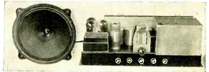
General view of the newest Silver-Marshall creation—the 728 S-W all-wave superheterodyne, fitted with automatic volume control and a separate oscillator for receiving short waves.
