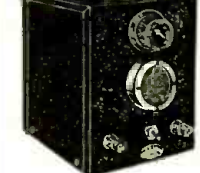
Excellent suited for P. A. work. Inter-communication systems, etc. Comprises sensitive single-button microphone, microphone coupling transformer and battery, cut-off switch, gain control and output terminals. Put up in neat black crackle-finished metal case, equipped with convenient carrying handle. Measures 5"x6 1/2"x6 3/4". Will correctly match the input impedance of practically all type amplifiers. Easily connected to the broadcast receiver for home recording. Ship. wt. 10 lbs. No. 1654—Pre-Amplifier. Your Price $8.25
