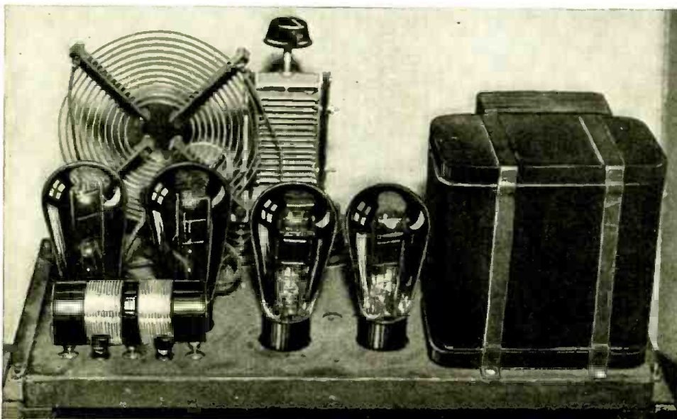
Above—The completed 30-watt transmitter which was built from the Kolster K-5 power amplifier.
